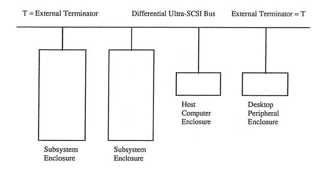
This sketch shows an environment with a limited number of enclosures, a reasonable bus length, terminators external to every enclosure, and a fairly static configuration.
