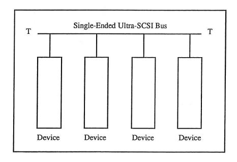
This sketch shows an environment with a fixed number of device slots, a very short bus, terminators external to every device, and a well-controlled electrical configuration. This would be useful in storage subsystem enclosures.
